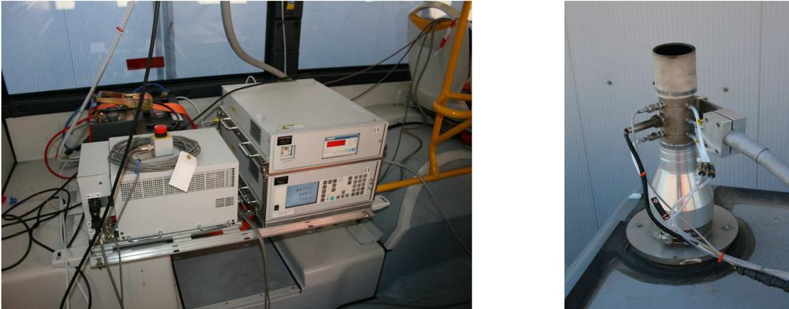
Figure 1 : on-board instrument: gas analyzer (a) and exhaust gas flowmeter (b)
